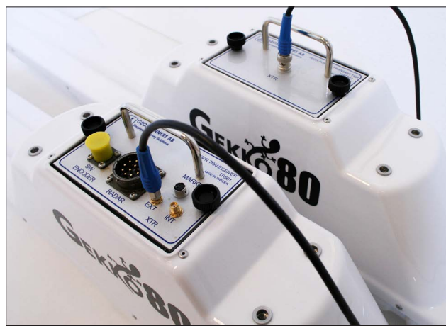
2. Two Gekko-80 antennas equipped with the proper plug-in electronics for bi-static mode.
