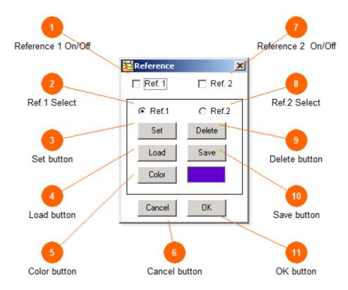
The reference setup button invokes a new window with all the options for setting reference functions. This is a useful editing tool when two or three different phase responses most be compared to each another.
