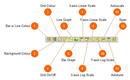
This toolbar contains controls that affect the way the spectrum data view presents the data. The options selected here are valid only during the processing and viewing of the imported file. The default values will be restored after importing another file.
