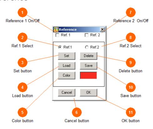
The reference setup button invokes a new window with all the options for setting reference waveforms. This is a useful editing tool when two or three different traces most be compared to each another.
