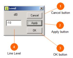
Use this dialogue box to select the level for the reference line on the spectrum data view.
