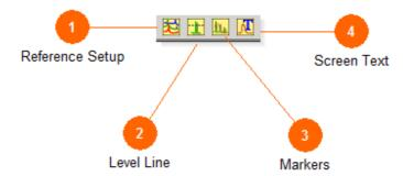
The editing tools provide an easy and fast way to add level lines, text, markers and reference spectrum lines to the existing spectrum plot.
