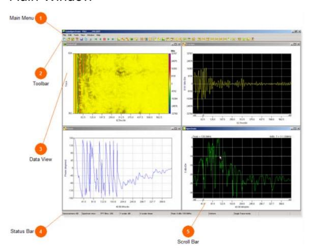
The main window of GaiaSpectrum® has the main menu, the toolbar, the data view or views and the status bar. The spectrum and o-scope data views have both a scroll bar that allows for moving the data back or forward in order to find troublesome areas.
