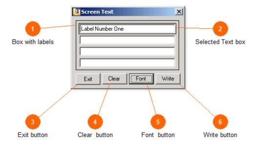
Dialogue box for entering and formatting labels to be displayed on the spectrum, o-scope, phase or waterfall data view.
