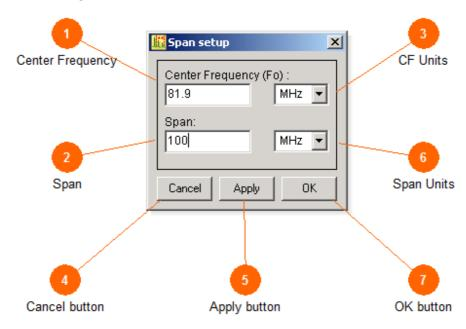
The span setup button invokes a new window that allows for selecting a portion of the spectrum function in the spectrum data view. In such a way it is easy to observe and measure a specific portion of the spectrum in a greater detail. If the span setup button is depressed then the spectrum data view shows the entire frequency span from zero to the maximum available frequency component.
