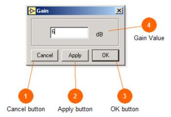
This dialogue box is used to enter the desired amount of amplification to apply to the current data set.
