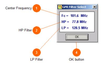
This window presents information on the recommended settings for the digital filters in ground penetrating radar systems.
