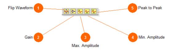
These are a set of automatic and semiautomatic measurement and editing tools based upon the waveform loaded in the o-scope data view.
