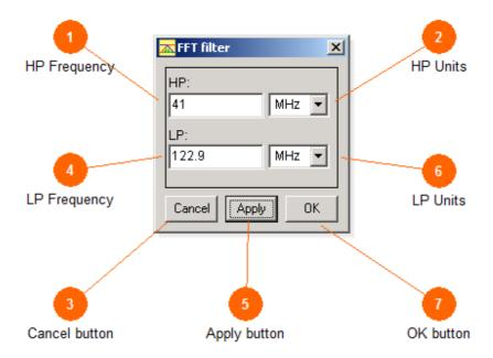
Enter in this dialogue box the low and high cut-off frequencies for the FFT filter. By combining these settings any kind of filter response can be achieved.
