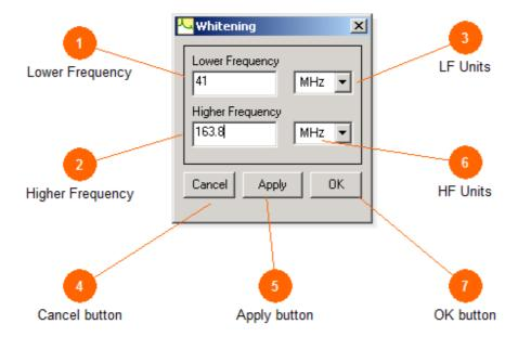
Enter in this dialogue box the values for the lower and upper frequencies of the desired pass-band to apply whitening.
