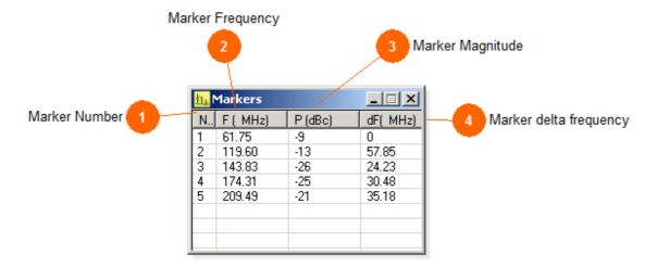
This window displays all the relevant information on the markers the users has set up in the spectrum data view.
