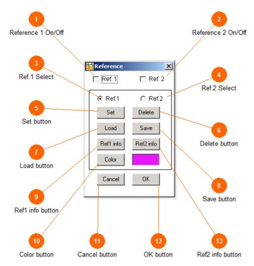
The reference setup button invokes a new window with all the options for setting reference spectrum lines. This is a useful editing tool when two or three different spectrum most be compared to each another.
