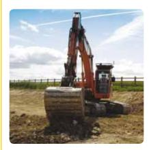
The EZiDIG system can now fully integrate with selected Leica PowerDigger machine control systems, providing the added functionality of cable location with precision excavator guidance.
