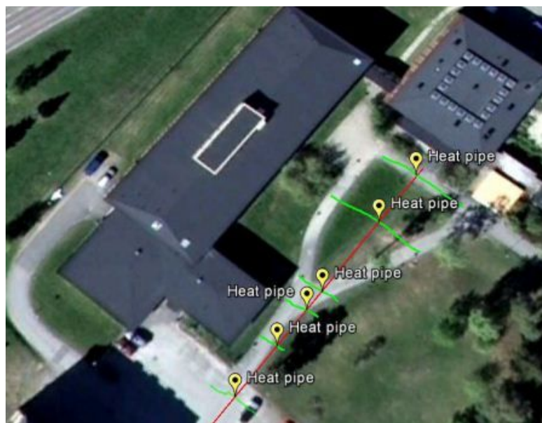
Picture 10. Google earth output of the located and positioned heat pipe
